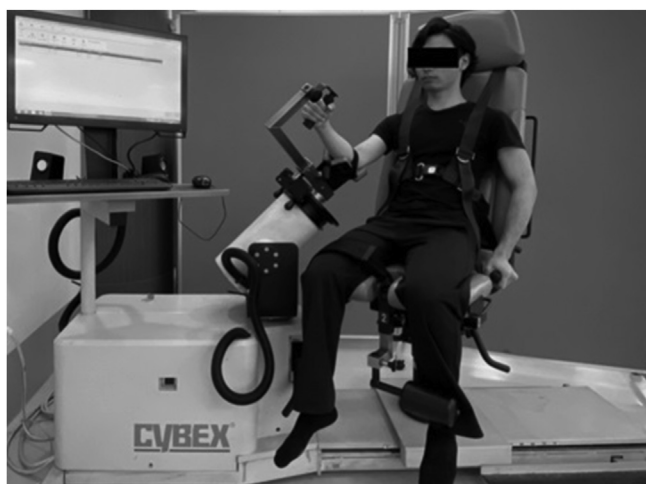
Fig. 3. Measurement of the muscle strength. The peak torque of the external shoulder rotator was measured using an isokinetic dynamometer, in a seated position with the arm in the scapula plane (45° of abduction, 30° of flexion).
